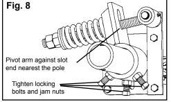
8. Tension the blade to the belt. Rotate the blade until it contacts the belt. While holding the spring bushing flat on the torque arm, rotate the torque arm until the pivot arm is against the end of the slot nearest the pole. Tighten the locking bolts and jam nuts on the torque arm (Fig. 8). NOTE: The torque arm should be up against the mounting plate.
