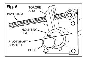
6. Install the QMT spring tensioner. Remove the adjusting nuts and springs from the pivot rod. Insert the pivot arm through the slot in the torque arm. Slide the torque arm onto the pole end (be sure the rotation of the arm is correct to tension the blade) and rotate it until the pivot shaft bracket lines up with the desired bolt holes (Fig. 6). Remove bolts, nuts and washers from mounting plate and reinstall through pivot shaft bracket and mounting plate.
