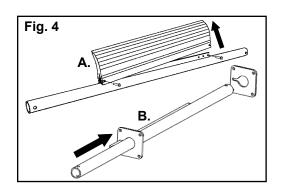
**4. Install the pole.** Remove both blade pins and blade from the pole and insert the pole in through the mounting plates (Fig. 4).
